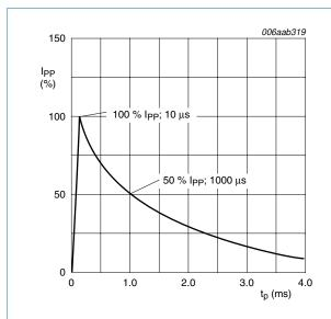
Fig 1.  $10/1000 \mu s$  pulse waveform according to IEC 61643-321
